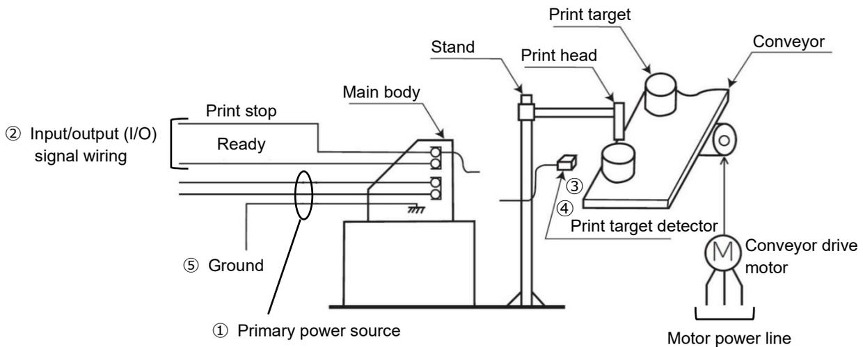
**Electric signal connection diagram**
