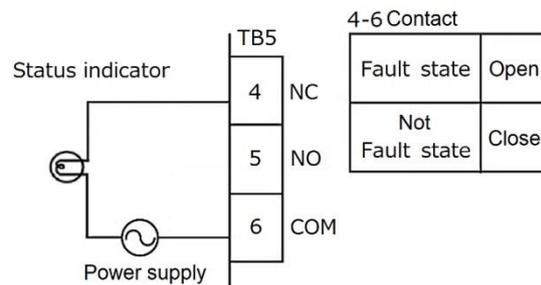
4.3.4.5. Warning Signal Output (Output via NPN Interface: Pin Number 13 on Terminal Block TB1, Relay Output: Pin Numbers 7 to 9 on Terminal Block TB5 \*TB5 IS OPTIONAL PARTS.)
