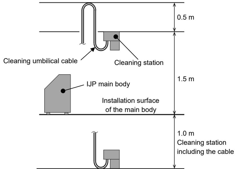
**Installation positions of Cleaning Station and cleaning umbilical cable**
