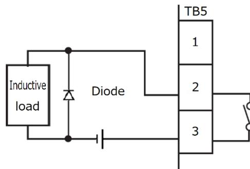
Use a diode that has a reverse withstand voltage 10 times or more the voltage used and a forward current more than the load current.
