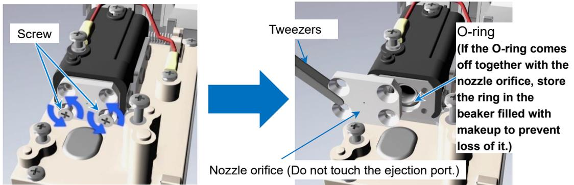
(d) Put the removed nozzle orifice into the beaker filled with makeup and clean it.
