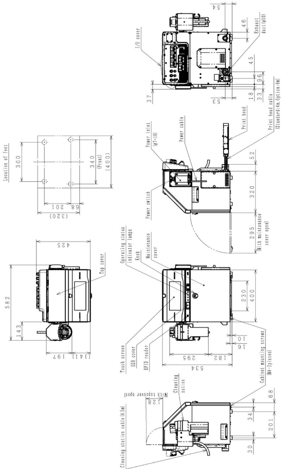
**Model UX2 IJ Printer, main body with Safe Clean Station dimensional drawing (Safe Clean Station and Handle are mounted)**
