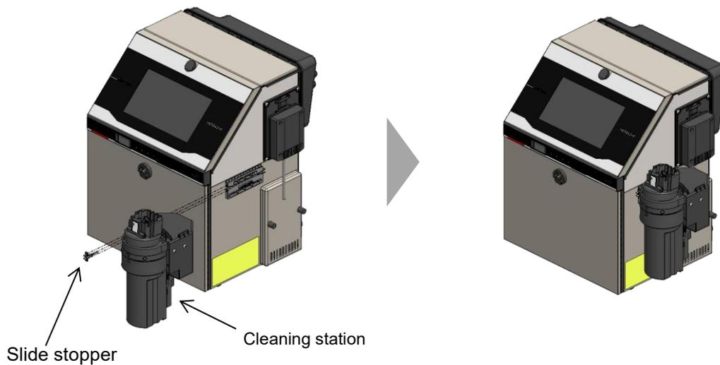
This completes the installation of the Cleaning Station.
