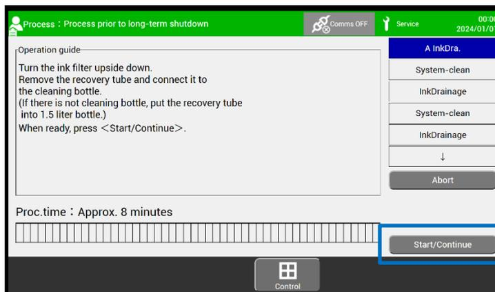
**[Process prior to long-term shutdown] screen (circulation system cleaning)**
