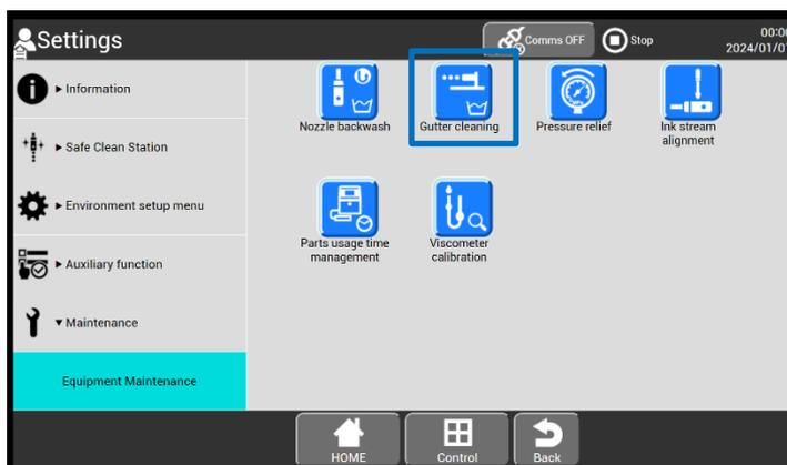
**[Maintenance(Equipment Maintenance)]screen (selecting [Gutter cleaning])**
