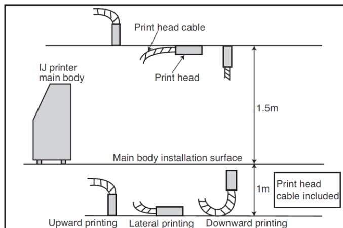
**Installation position of end of print head (for 0 to 45°C)**
