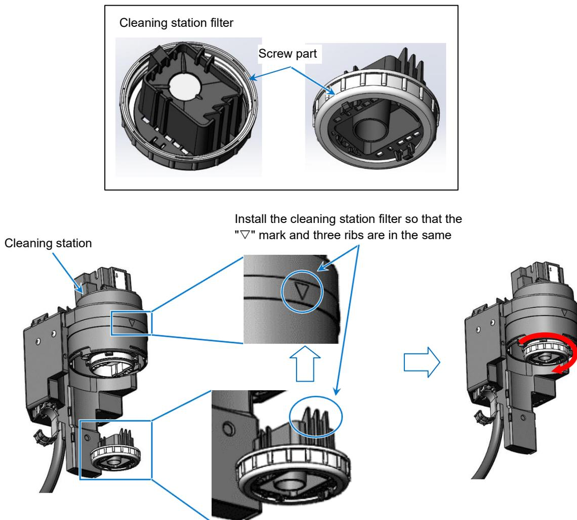
How to install cleaning station filter
