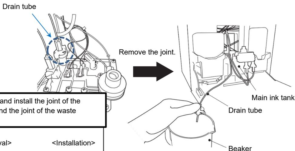
How to remove and install the joint of the recovery tube and the joint of the waste solution bottle
