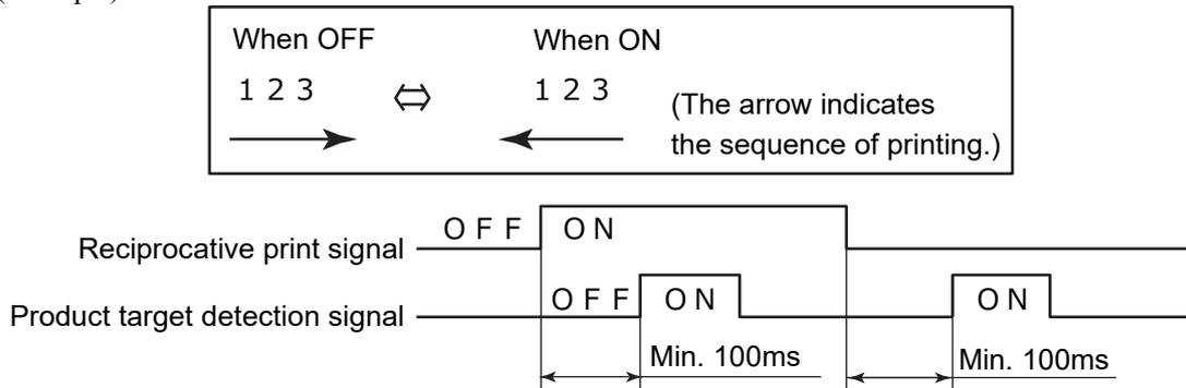
\*When the user environment setup item "Change Character Orientation" was set to "Reverse direction printing", provide a minimum interval of 100ms up to input of the print target detector signal after changeover (ON→OFF, OFF→ON) of the reciprocative printing signal.
