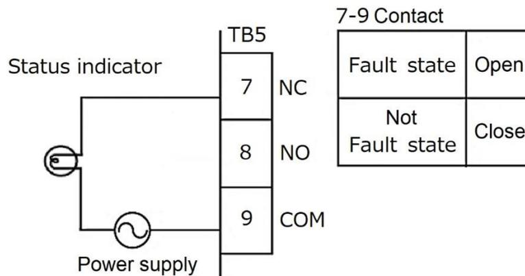
For warning and fault output, each of NO and NC contacts supports a capacity of up to 100 VAC/0.5 A or 30 VDC/1 A. For the use of the unit under a load larger than the capacity, interpose another relay in the connection.
