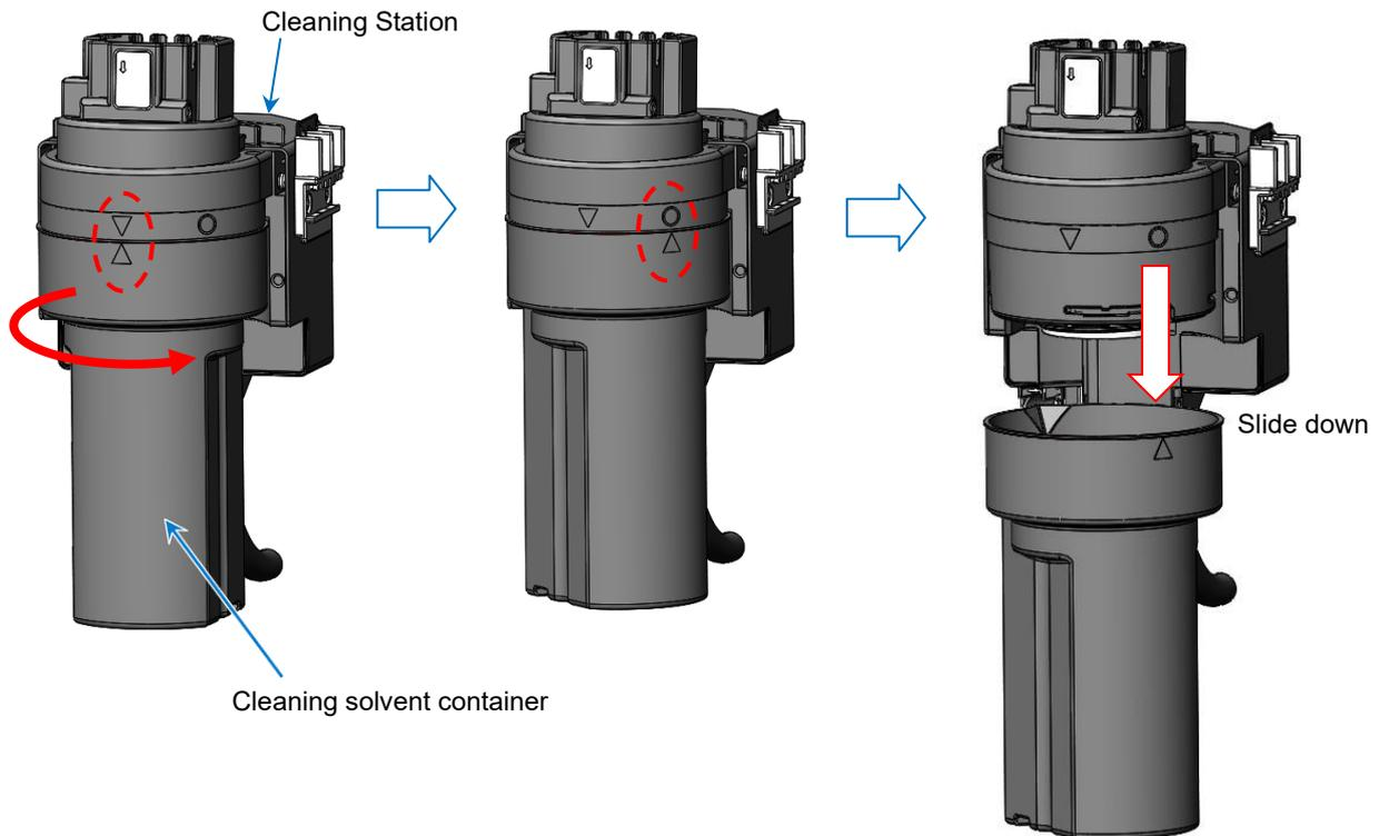
**How to remove cleaning solvent container**
