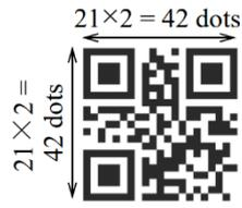
1 Cell = 2 dots (Vertical 2 dots × Horizontal 2 dots)
