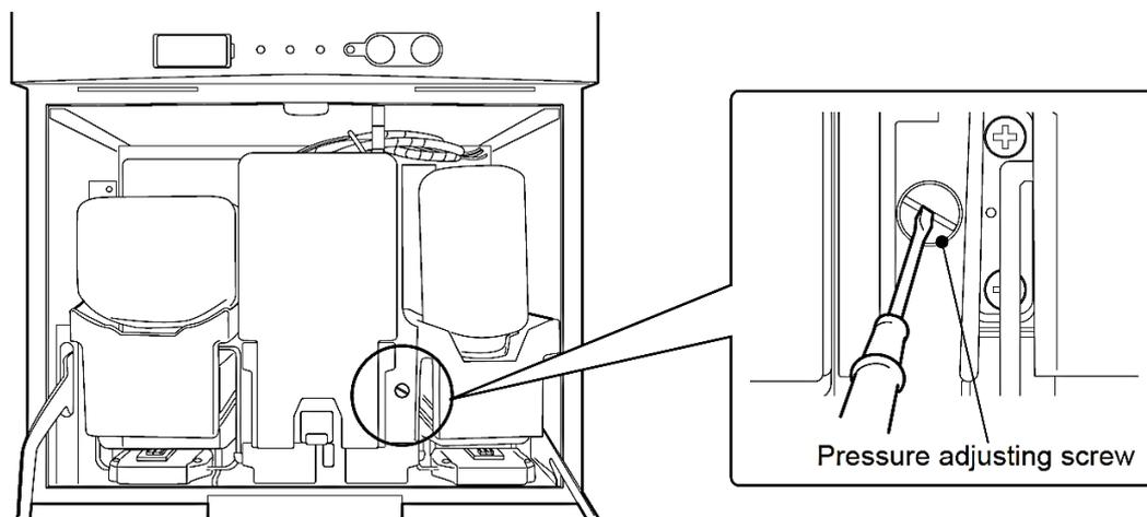
To raise the pressure : rotate clockwise.
