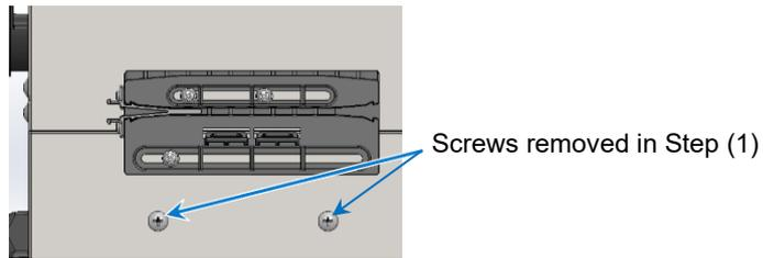
(6) Align the Slide base with the grooves of the slide block, and slide the jig to install it.
