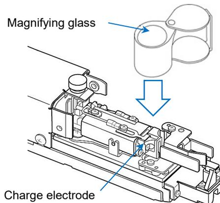
**Diagram of observing ink drops (using magnifying glass)**
