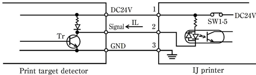
The input circuit of the IJ Printer is a current drive load to the output circuit of the print target detector, and when the output transistor  $T_r$  of the print target detector is switched on, it becomes an input of the start print signal.
