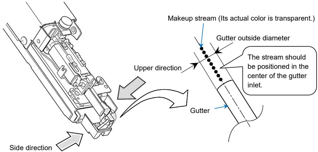
If the stream is not in the center of the gutter, perform the nozzle backwash again.
