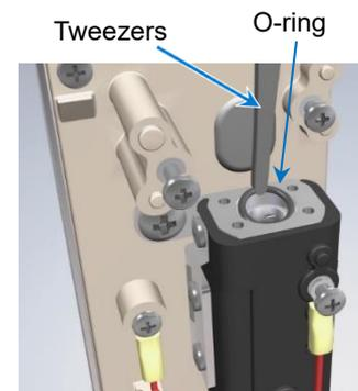
(b) Pour a few drops of makeup into the O-ring from the cleaning bottle to make it easier to insert the nozzle orifice.
