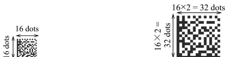
1 Cell = 1 dot (Vertical 1 dot × Horizontal 1 dot)      1 Cell = 2 dots (Vertical 2 dots × Horizontal 2 dots)
