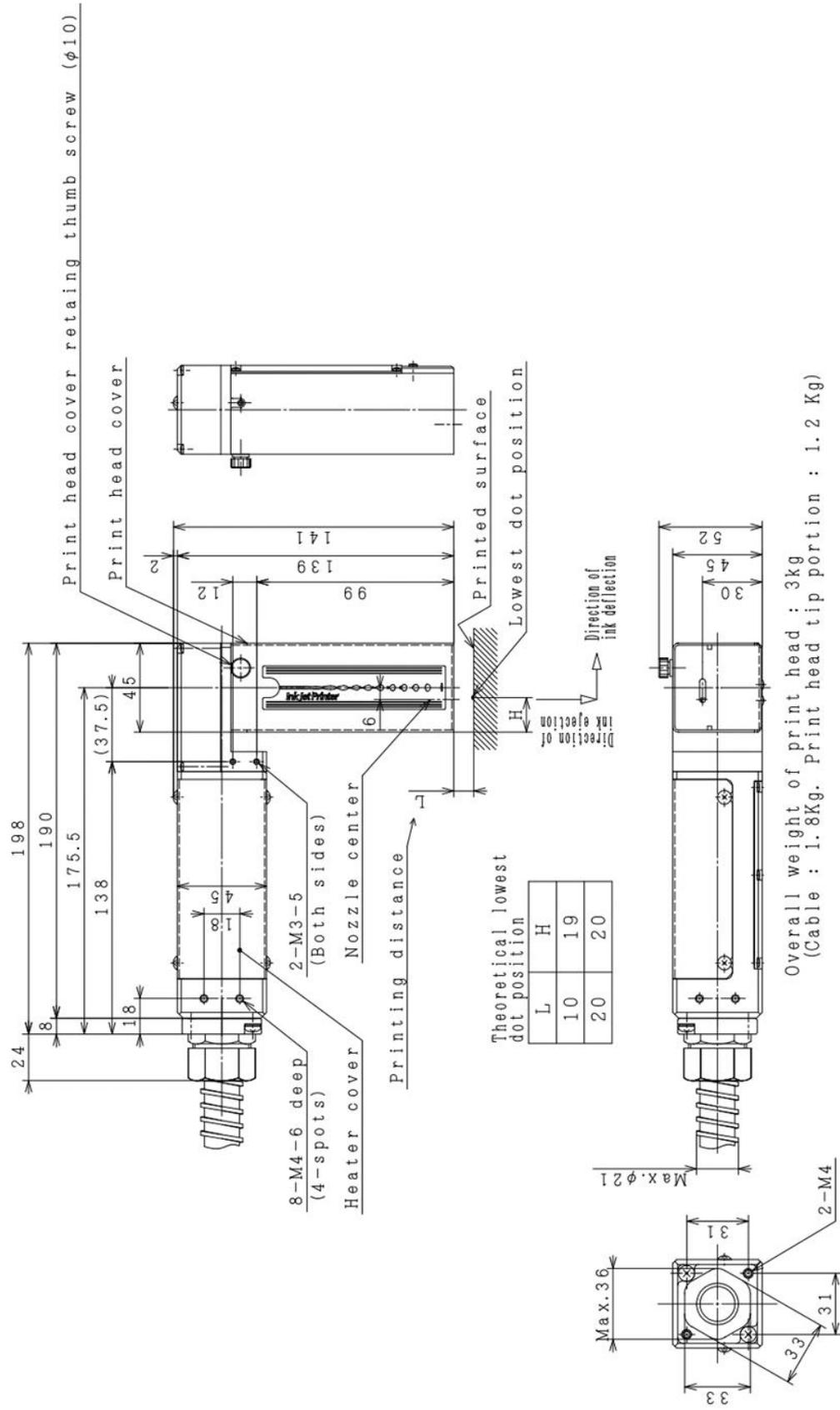
Model UX2-D160W IJ Printer, 90 Degree print head dimensional drawing
