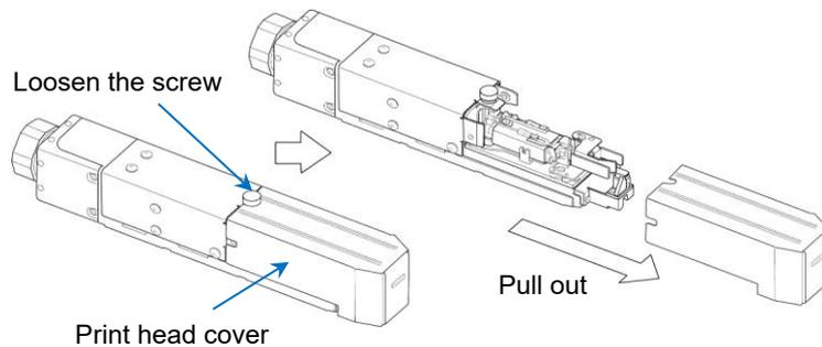
**Diagram of removing print head cover**
