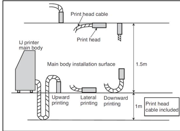
**Installation position of end of print head (for 45 to 50°C)**
