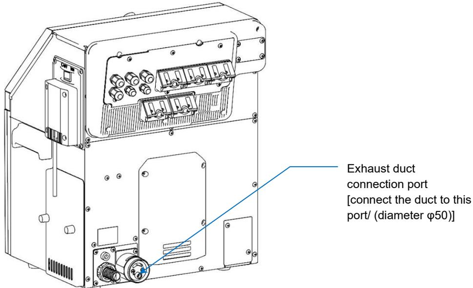
**Exhaust duct connection port**
