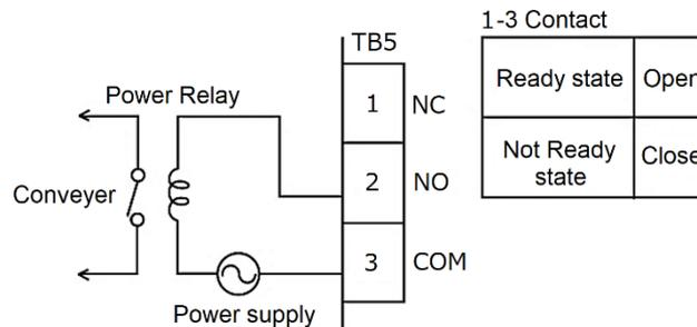
Each of NO and NC contacts supports a capacity of up to 30 VAC/0.5 A or 30 VDC/1 A. For the use of the unit under a load larger than the capacity, interpose another relay in the connection. When the load is an inductive load such as a motor or a relay, counter electromotive force may be generated, which may shorten the life of the contact. Be sure to protect the contact. Typical contact protection methods are described below.
