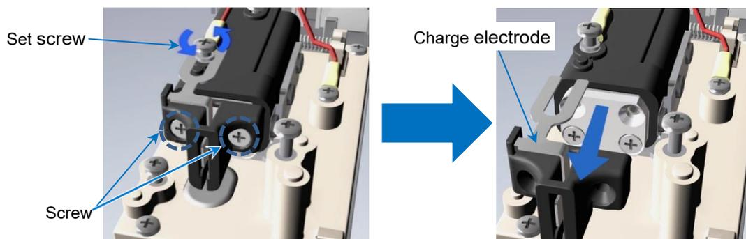
(c) Loosen the set screw, remove the two screws of the nozzle orifice, and remove the nozzle orifice.
