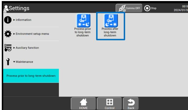
**[Process prior to long-term shutdown] screen (selecting [Process after long-term shutdown])**
