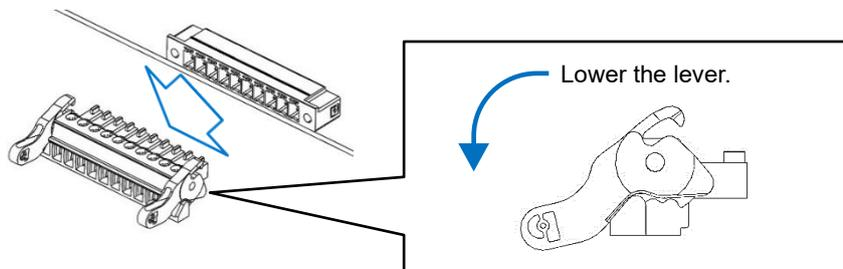
[Connecting to the external connection terminal block (TB1 and TB2 on the EZJ144 board)]
