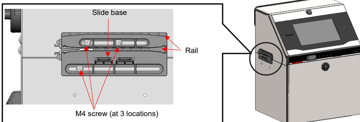
(5) Attach the M4 screws removed in Step (1) to their original positions.
