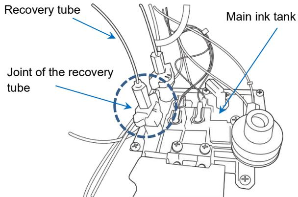
How to remove and install the joint of the recovery tube and the joint of the waste solution bottle
