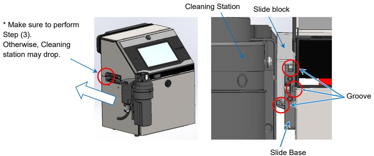
(7) Install the cleaning unit stopper (one piece) on the Slide base, and fix the Cleaning Station with the supplied M3 screws.
