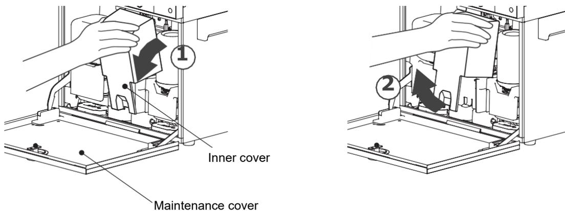
**Procedure for removing inner cover**
