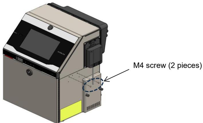
(3) Use attached M4 screws (4 pcs) to fix the Slide base to the main body.
