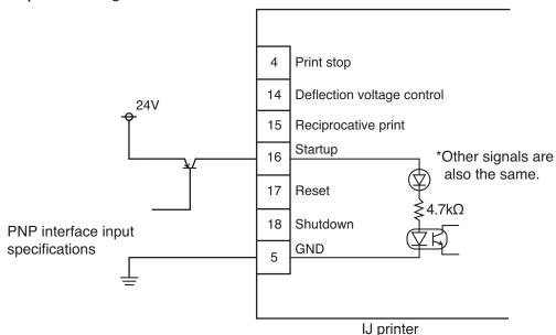
• Each input is activated when contact ON.
