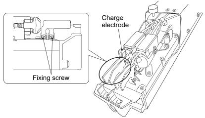
(b) Remove the two screws holding the charge electrode and remove the charge electrode.
