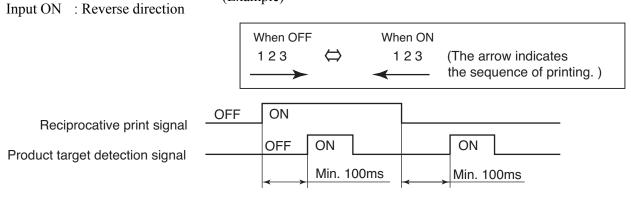
\*When the user environment setup item "Change Character Orientation" was set to "Reverse direction printing", provide a minimum interval of 100ms up to input of the print target detector signal after changeover (ON→OFF, OFF→ON) of the reciprocative printing signal.
