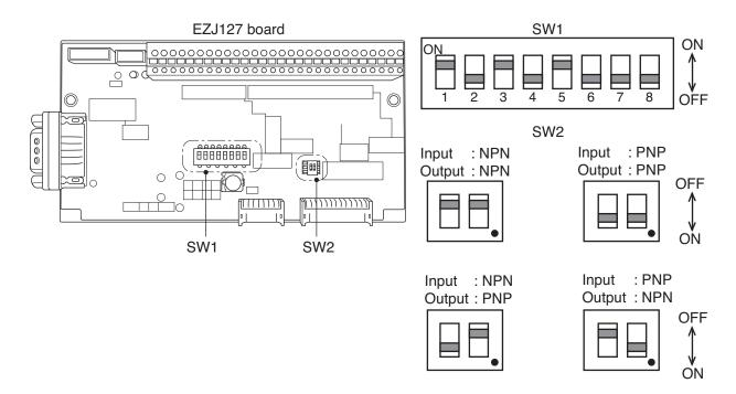
(Precautions when using combination of NPN/PNP interfaces)
