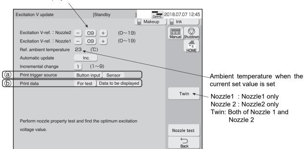
• When "Print start adjust mode" is set to "Enable" on User environment setup screen, "Nozzle switching button" on screen at middle right shall be set to "Twin".
