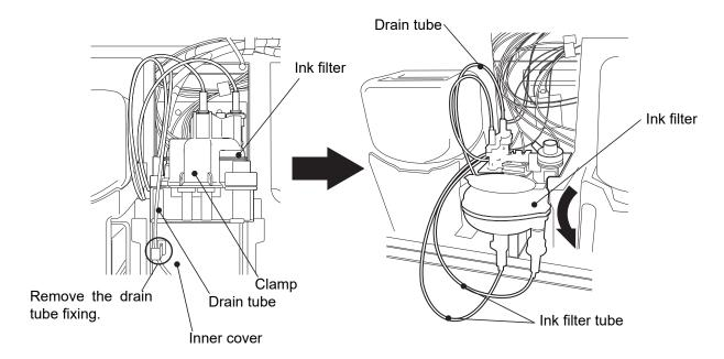
• Disconnect the drain tube from the main ink tank and insert it into the beaker. \*Set the beaker at a position lower than the main ink tank.
