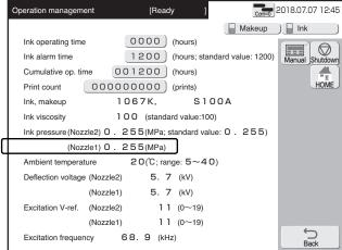
Check the displayed ink pressure value of nozzle 1. If there is a difference of 0.010 or more from the standard value, adjust the pressure to the standard value ±0.002 with a flat-blade screwdriver.
