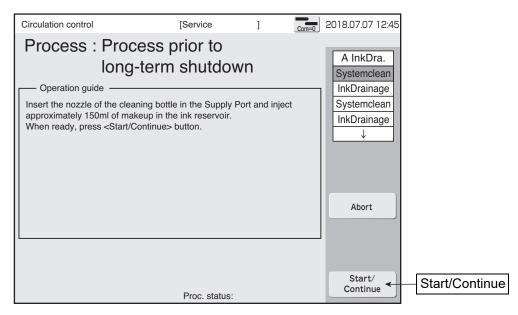
(a) Insert the nozzle of the cleaning bottle in the supply port and Inject approximately 150ml of makeup int the ink reservoir.
