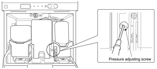
To raise the pressure : rotate clockwise.
