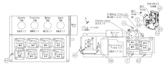
Fig.8-5 Model UX-D860 Tube connection
