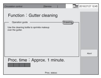
• Pour makeup onto the gutter.
