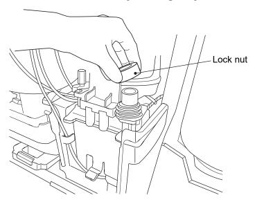
3 Remove the filter case upward and set the new Mini filter.
