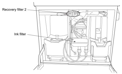
Remove the lock nut of recovery filter 2 by turning it by hand.
