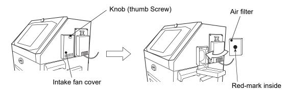
3 Set the intake fan cover. (Turn the knobs until the intake fan cover comes into contact with the printer.)
