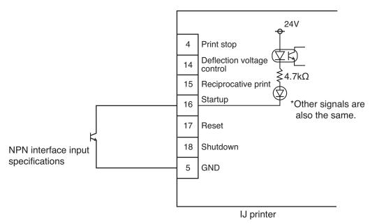
•Each input is activated when contact ON.
