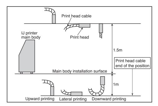
(10) When using the printer for upward or lateral printing, ensure that the rising print head cable upper end is positioned not more than 0.5 m above the print head.
