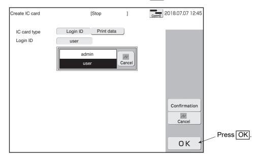
When the message, "Create IC card is in progress. Please pass IC card over the reader." is shown, pass the IC card over the reader on the IJ printer main unit (Fig. 1).
