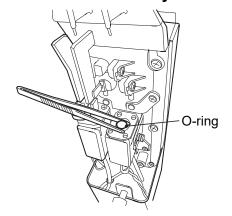
(b) Use the cleaning bottle and splash a few droplets of makeup on the O-ring.
