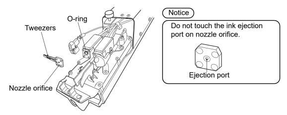
The O-ring may detach from the nozzle orifice at this time. If it does, put the O-ring in a beaker with makeup ink and take care not to lose it.
