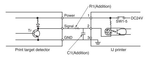
If R1=1kohm (0.5W) and C1=1micro farad /25V, the CR time constant=1ms. If R1=1kohm (0.5W) and C1=1micro farad /25V, the CR time constant=1ms. The filter could eliminate a several hundred micro-seconds of noise. If you need to eliminate bigger noise, add an additional capacitor in parallel with C1.
