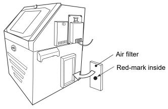
4 Set the intake fan cover. (Turn the knobs until the intake fan cover comes into contact with the printer.)
