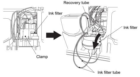
• Disconnect the recovery tube from the main ink tank.
