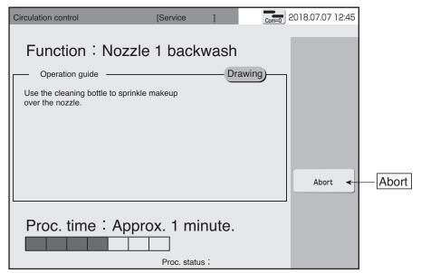
3 Suction begins automatically. Sprinkle the nozzle orifice with makeup.
