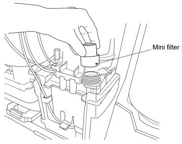
4 Set the new filter case and fix it with the Lock nut.
