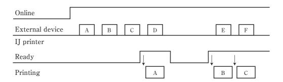
(Example 3) When offline is restored during normal operation, and printing is subsequently performed in standard mode:
