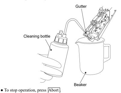
3 Cleaning ends in about 1 minute and the screen returns to the Circulation control screen.
