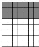
• For pattern data composition purposes, the data is arranged in successive order, beginning from the bottom left, from bottom to top and from left to right.
