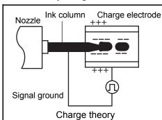
The ink drops are electrically charged by impressing a voltage between the charging electrode and ink column as shown at the left.
