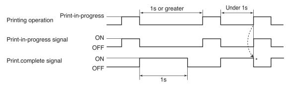
\*When the next printing operation started within 1 second, turned OFF at the stage at which the printing operation started.
