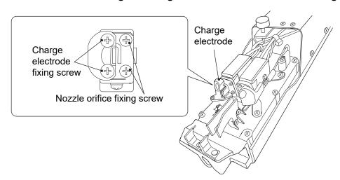
(c) Remove the two screws holding the nozzle orifice.
