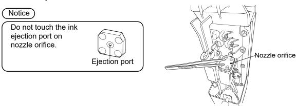
(d) Remove the nozzle orifice once and make sure that the O-ring has been installed.
