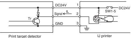
When the IJ printer input circuit is a current drive load for the print target detector output circuit and output transistor Tr of the print target detector is ON, it becomes the print start signal input. Use an output transistor Tr which satisfies the following specifications (NPN/PNP):
