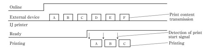
(Example 2) When status is restored to that other than ready during normal operation, and printing is to restart in ready status:
