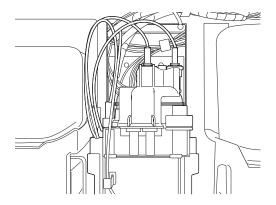
2 Tilt the ink filter the front and pull out the recovery filter 2.
