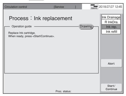
Follow the on-screen instructions to return the recovery tube to its original position and press Start/Continue.
