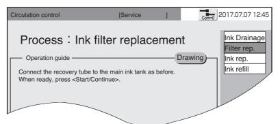
\*1 Clean the connection part at the tip of the recovery tube well with makeup before connecting to its original position.
